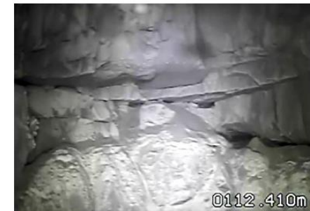
Figure 28: Fissured rock at a depth of 112,4 MBGL. Side view.
