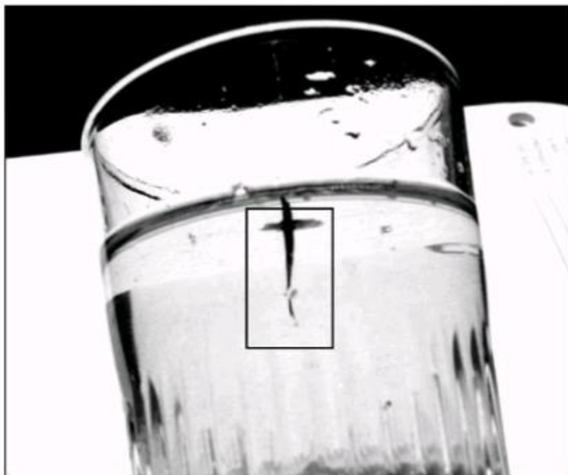
Figuur 4 Dense nonaqueous phase liquid tar droplet suspended at the water surface due to surface tension. Tar droplet floating at water surface is approximately 1 cm long and 0.3 cm wide at water surface, outlined in the box. Droplet shaped like a roofing nail; reflection of tail of the tar droplet appears to extend upward. Tar droplet fell through water column when surface tension was disrupted
